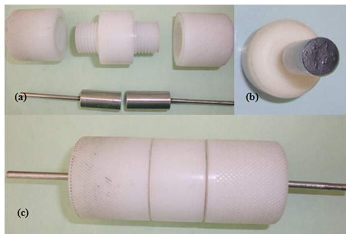
**Fig.1: (a) Test cell with two stainless steel electrodes (b) Prepared electrodes for testing (c) Final supercapacitor assembly**
