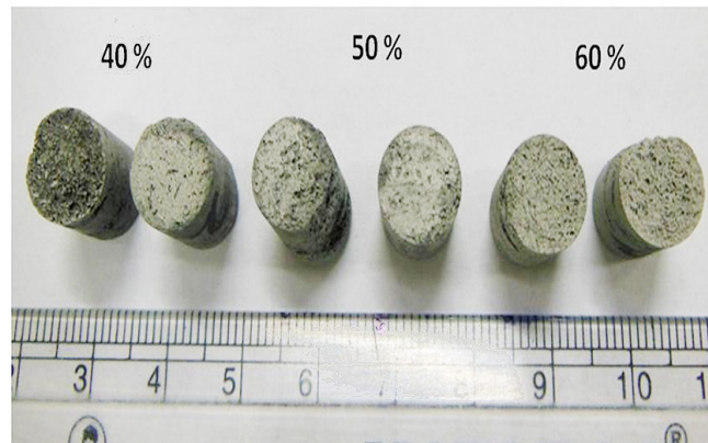
Fig. 5: Sintered stainless steel foam samples with varying porosity processed using acicular crystals of urea
