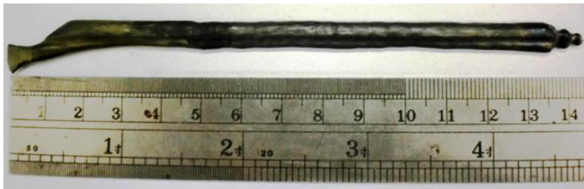
Fig. 6: Si crystal (~14.4 cm long) with nearly constant width grown by proper adjustment of gas flows (initially non-uniform up to 1.5 cm)
