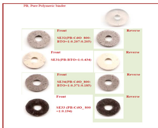
Fig. 4: Figure 4(i) shows our Annular Samples for 700MHz to 3GHz EMI shielding measurements with the Vector Analyzer.
