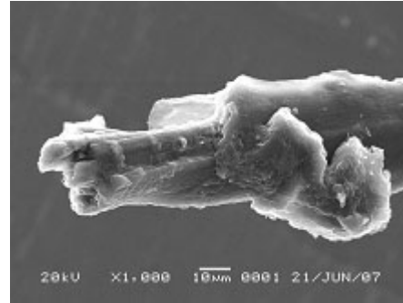
(a) Ramie-Green1-epoxy shows fiber pull-out and there is no epoxy still stuck on the fiber end surface(right). The embedded fiber seems to be pull-out easily from the matrix (left).
