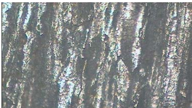
Fig. 4: Micrograph of mild steel surface attacked by 0.5M HCl solution with 48 h immersion at 25°C
