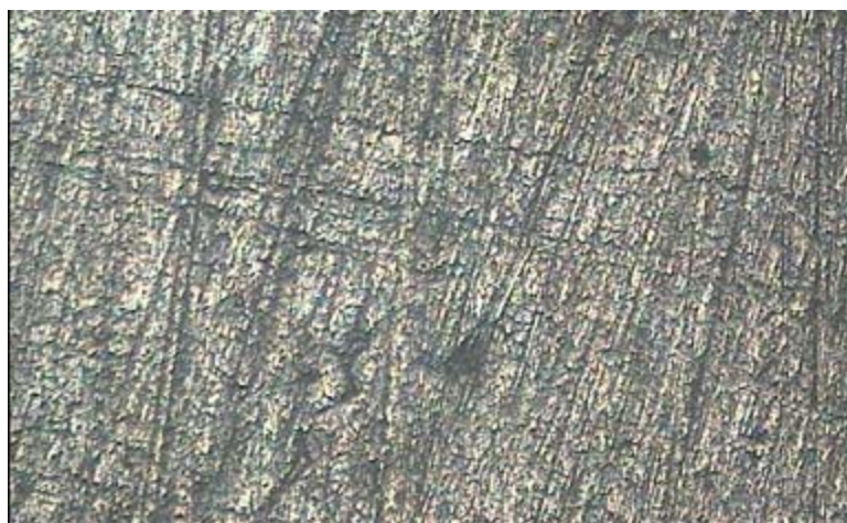
Fig. 5: Micrograph of mild steel surface attacked by 0.5M HCl solution with 48 h immersion in the presence of 250 ppm CTMAC at 25°C
