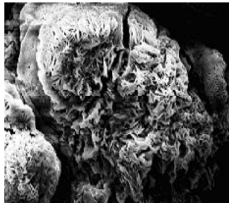
Fig. -10: Scanning Electron Micrograph of Mild Steel in presence of 1000 ppm[ N-( 3- Methylthio-5-acetamido-1,2,4-thiadiazolyl ) cytosine ] in 1M H 2 SO 4 at 2000
