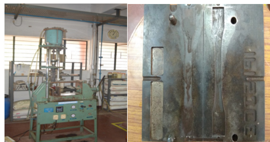
Fig. 4: injection moulding machine with mould cavity
